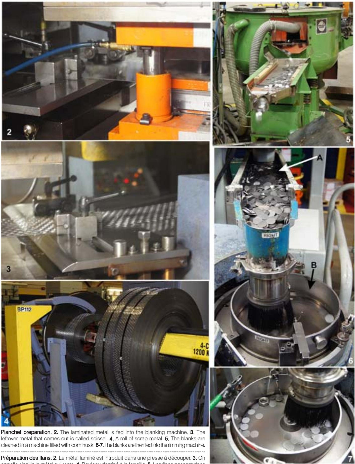
**Planchet preparation.** 2. The laminated metal is fed into the blanking machine. 3. The leftover metal that comes out is called scissel. 4. A roll of scrap metal. 5. The blanks are cleaned in a machine filled with corn husk. 6-7. The blanks are then fed into the rimming machine.
